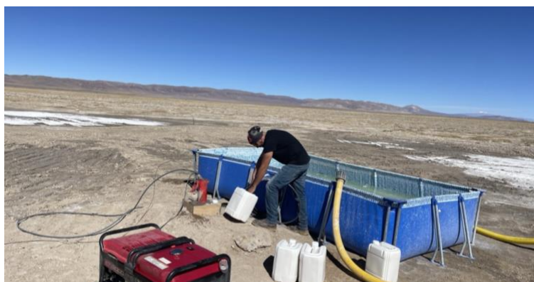
Figures 4 and 5: Photos of Collection of Brines for Field Testing Analysis and Chemical Assaying
