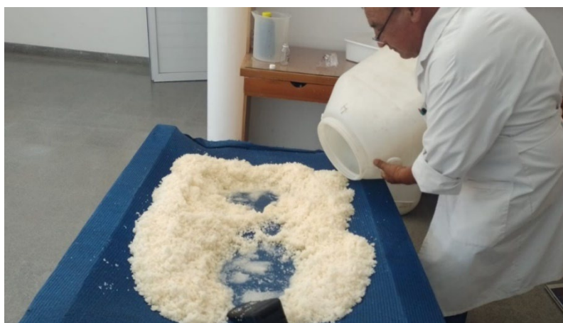
Figure 7: Salt Precipitation Stage, with concentrated brine separate from Salts
