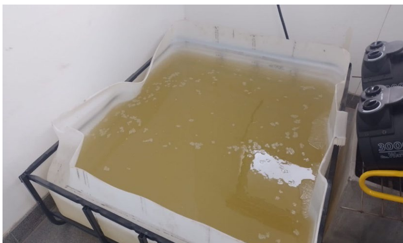
Figure 6: Primary Evaporation Stage of Solaroz Brines
