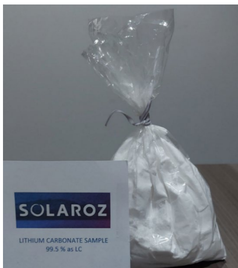
Figure 8: Final Battery Grade 99.5% Lithium Carbonate produced from the Solaroz Brine
