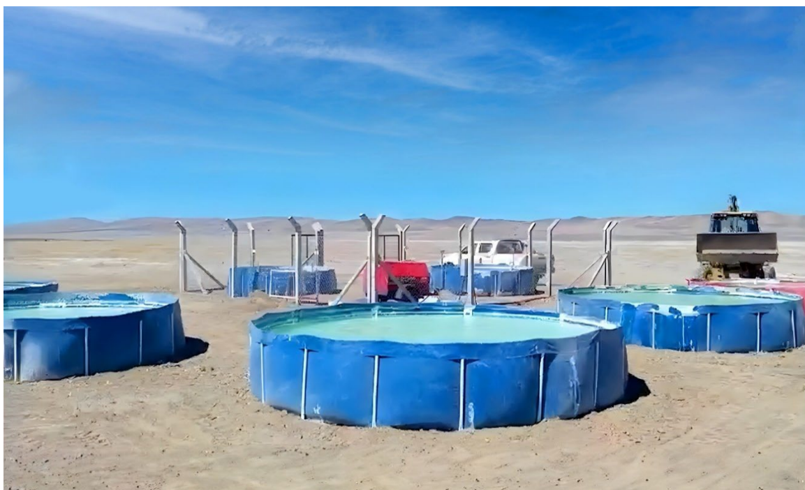
Figure 9: Solaroz Lithium Brine Project site test evaporation ponds
