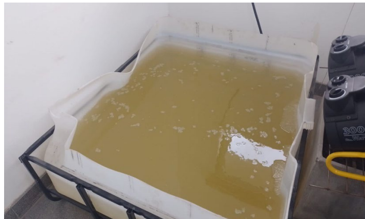
Figure 8: Primary Evaporation Stage of Solaroz Brines
