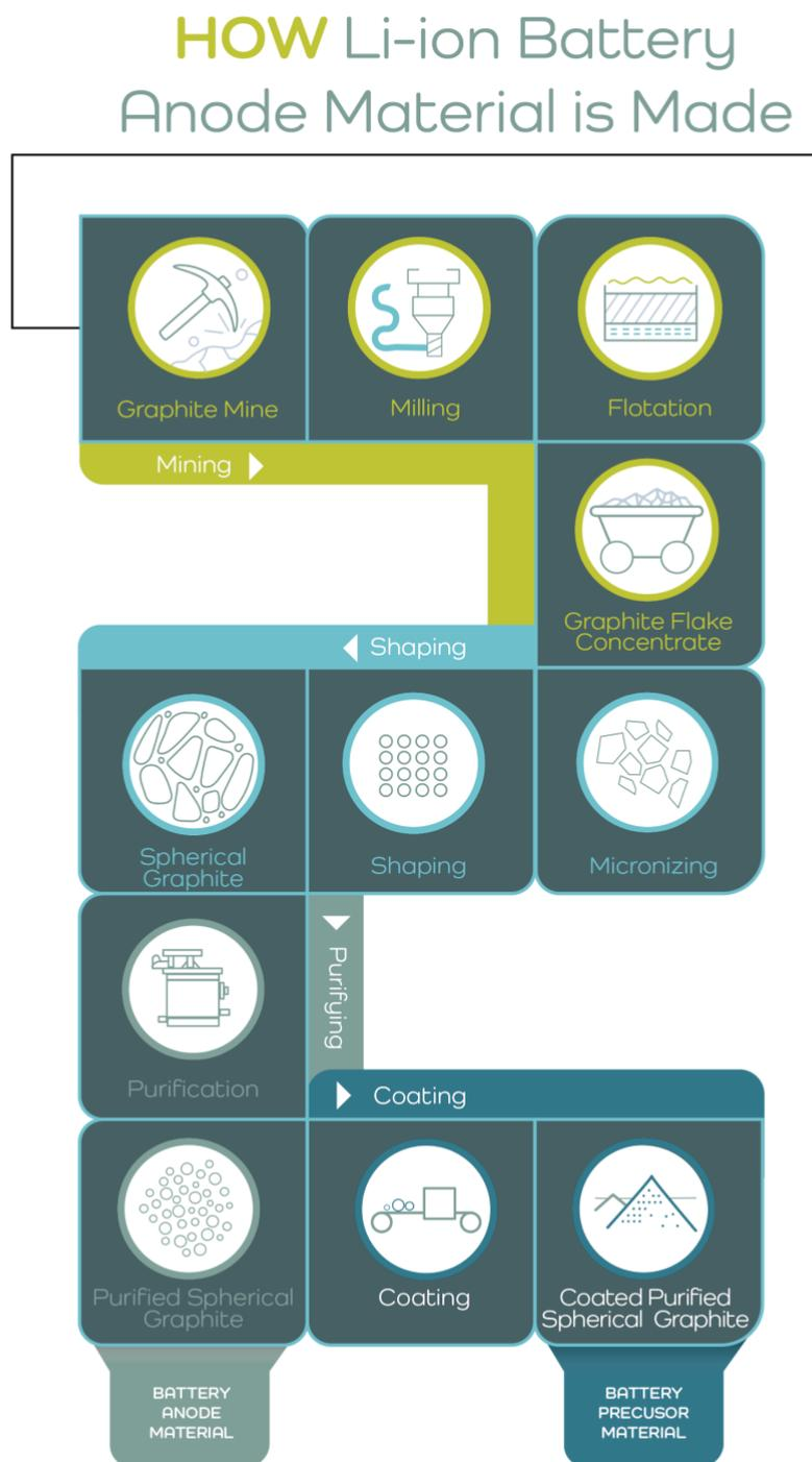
Figure 3: Illustrative Vertically Integrated Operations from Graphite Mine to Production of BAM
