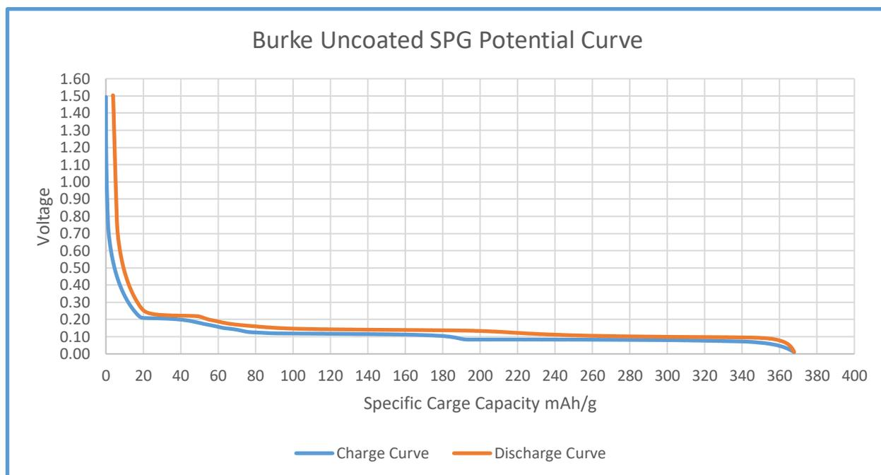
Figure 1: Potential Curve of the Swagelok®T-Cell (a conventional T-Cell battery used in battery research) using uncoated Burke SPG as the Anode
