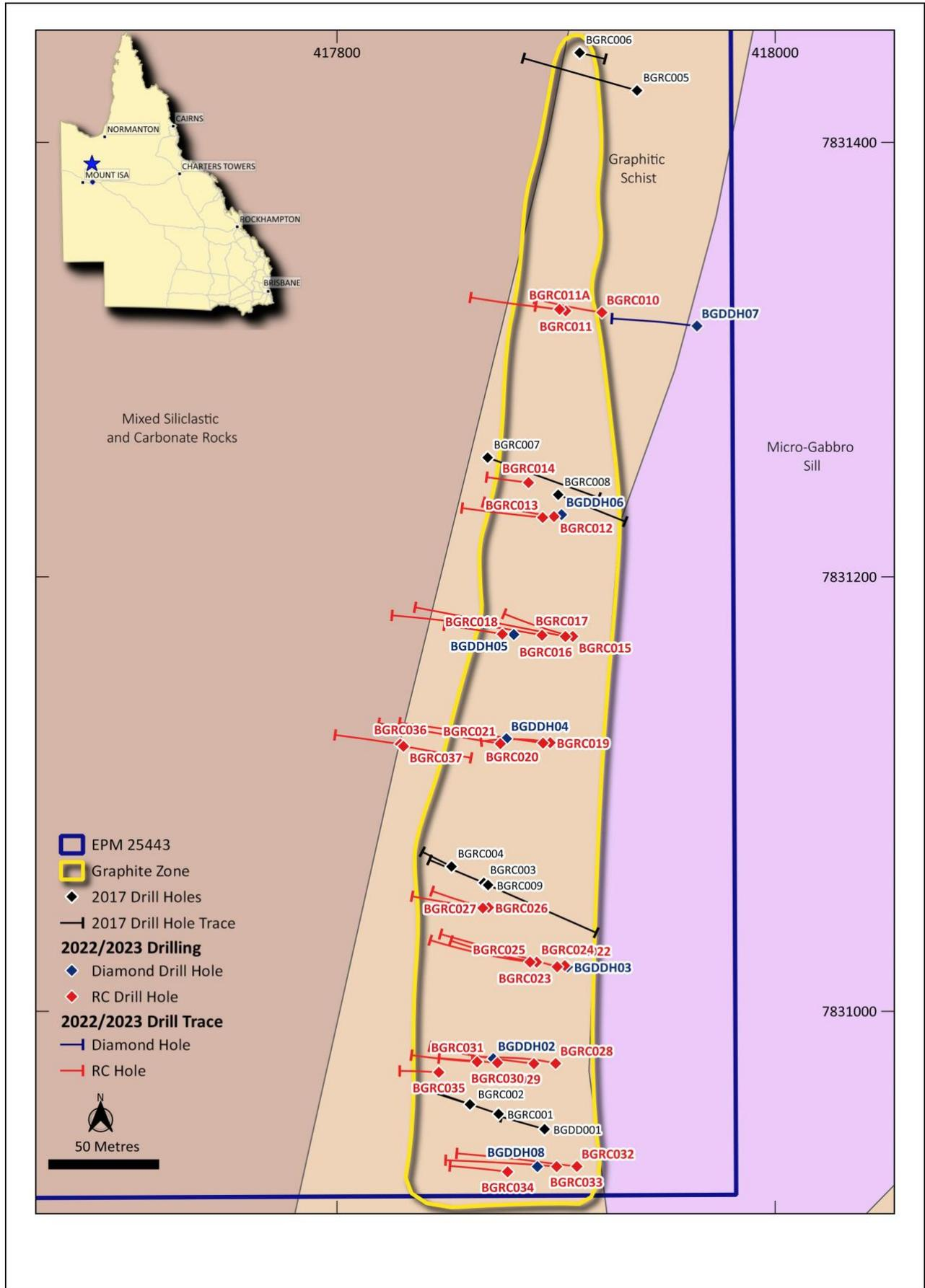
Figure 4: Location of RC (BGRC) and Diamond (BGDD) Drillholes
