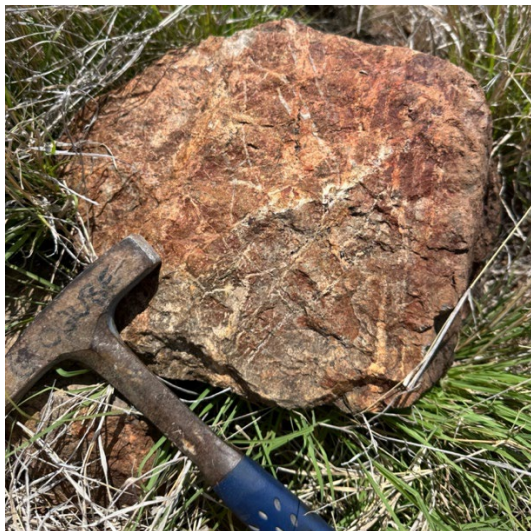
Stockwork quartz-potassium feldspar veining (at 217903mE, 7372231mN)
