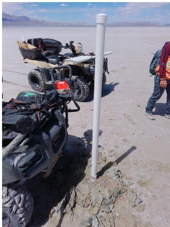
Figure 2: Hand Auger drill hole recently completed at White Plains Lithium Brine Project
