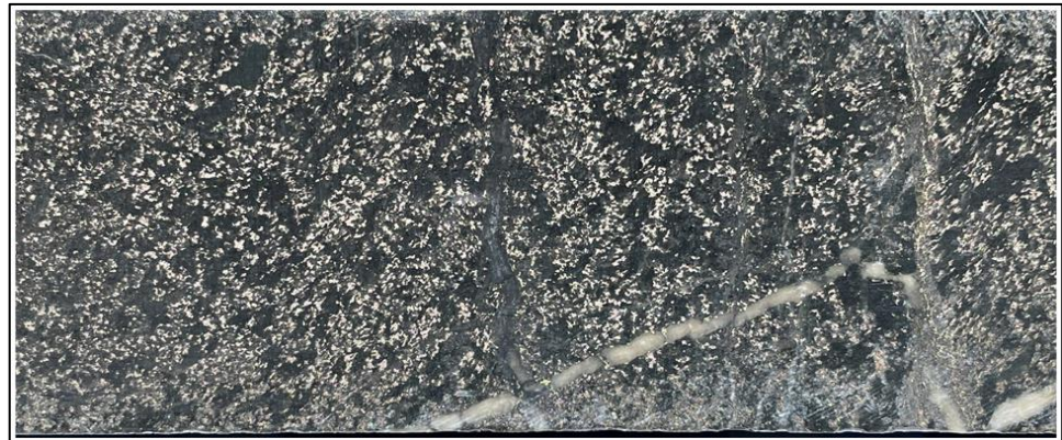
Figure 1: Silicified basal ultramafic with disseminated pyrrhotite/chalcopyrite and pyrite plus minor pentlandite (321.8m downhole in FOS21DD_003) – core width 50mm for scale
