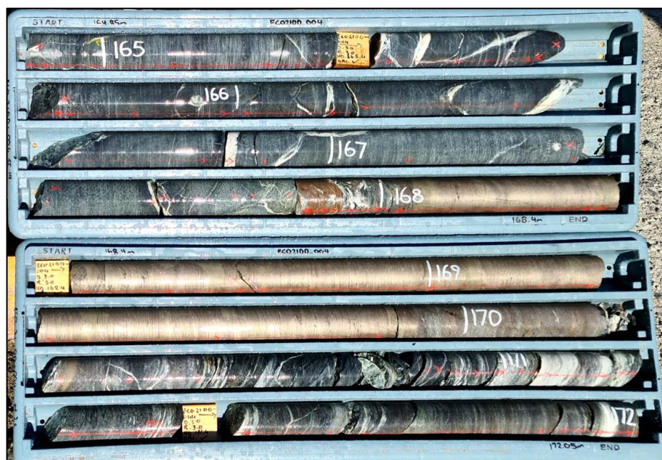
Figure 1 : Core from ECO21DD_004 - massive nickel sulphide zone from 168m downhole
