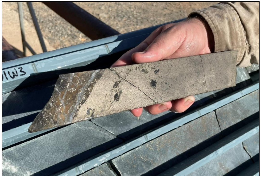
Figure 1: Diamond core with massive nickel sulphides from the third wedge daughter hole (from 504.58m)
