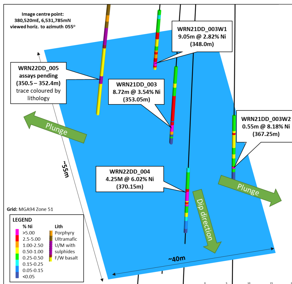
Figure 1: Perspective view of DHTM conductive plate showing WRN21DD_003 parent and the completed wedge holes (W1 & W2) and new surface holes WRN22DD_004 and 005.
