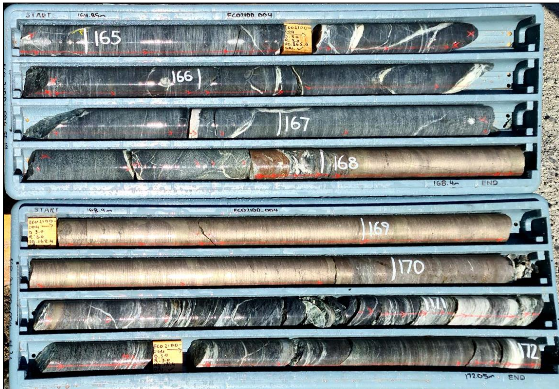
Figure 2 : Core from ECO21DD_004 - massive nickel sulphide zone from 167.85m downhole: 2.7m @ 10.72% Ni
