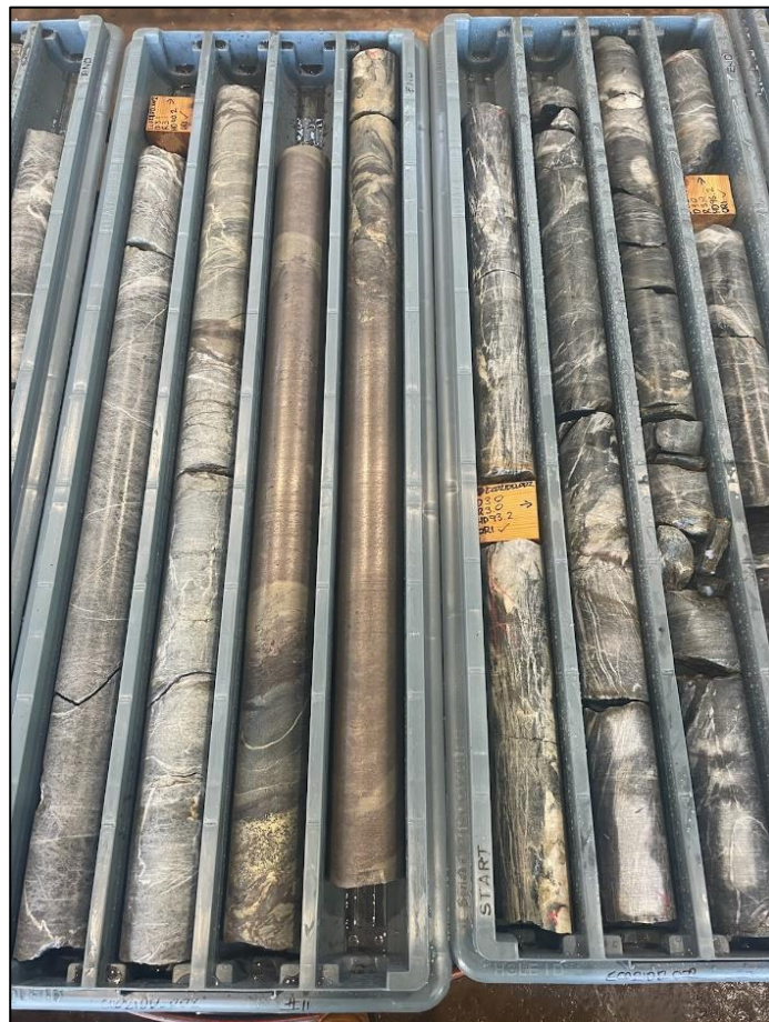
Figure 3: Core from ECO21DD_003 - massive nickel sulphide zone from 122.1m downhole: 2.15m @ 5.53% Ni
