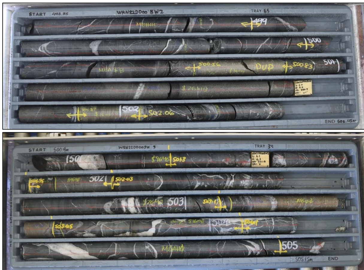
Figure 4: Core photos of Tray 65 from WRN22DD_008W2 (top) and Tray 34 from WRN22DD_008W3 (bottom) illustrating nickel sulphides intersected – see Annexure 3 for summary geological logs.
