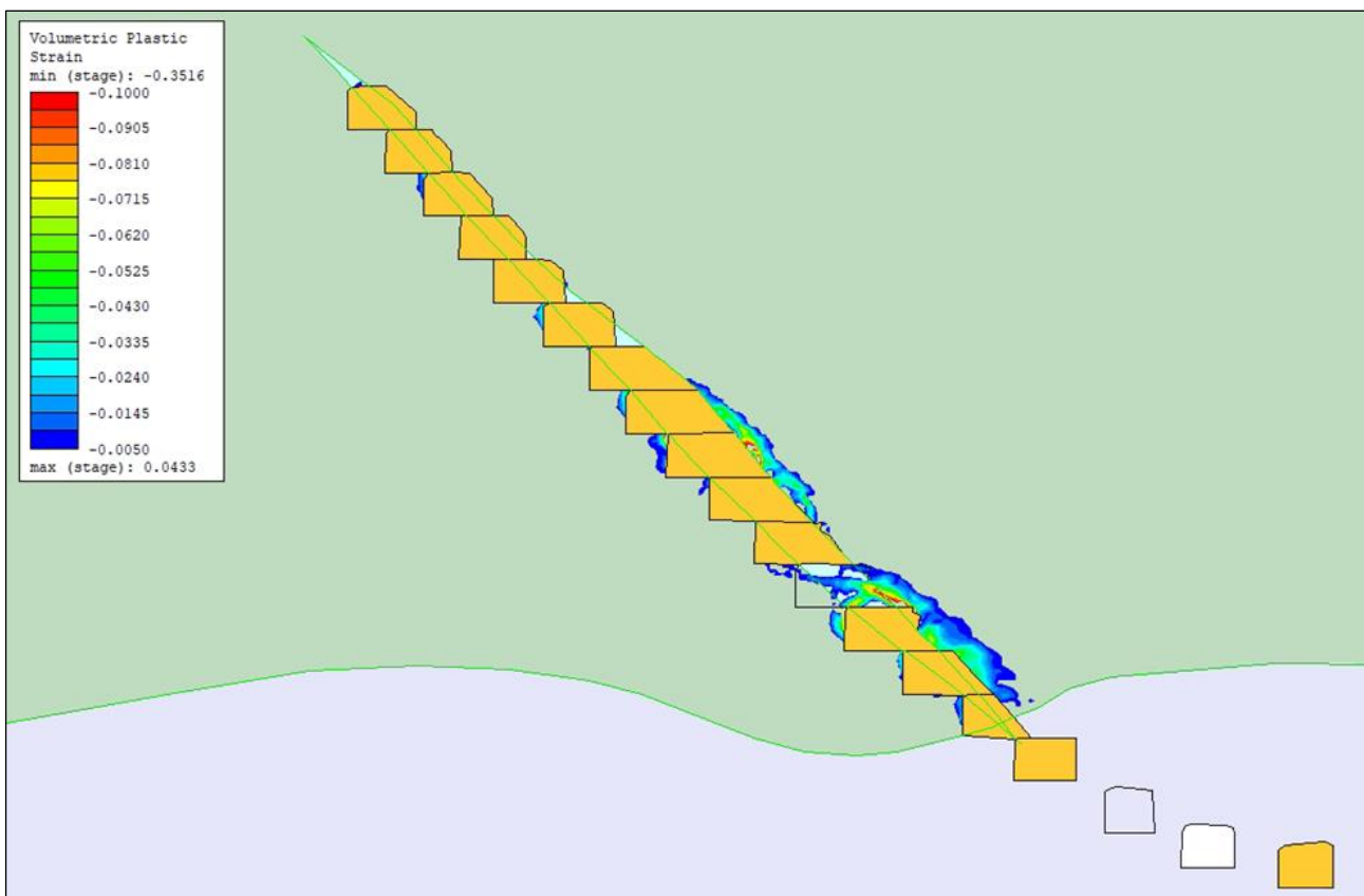
Figure 7: Numerical modelling indicated minor damage in hangingwall and sill pillar during final phases of stoping
