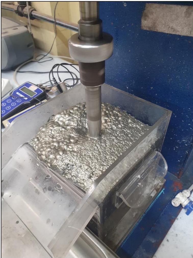
Figure 17: MOB02 flotation test in progress
