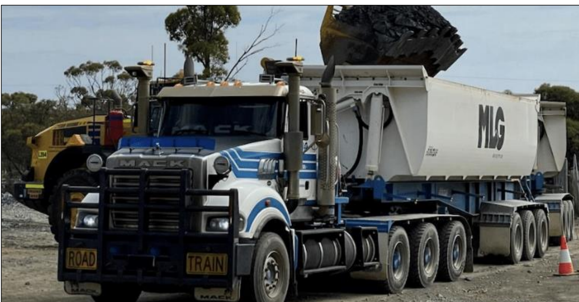
Figure 20: Typical road-train loading and haulage arrangement
