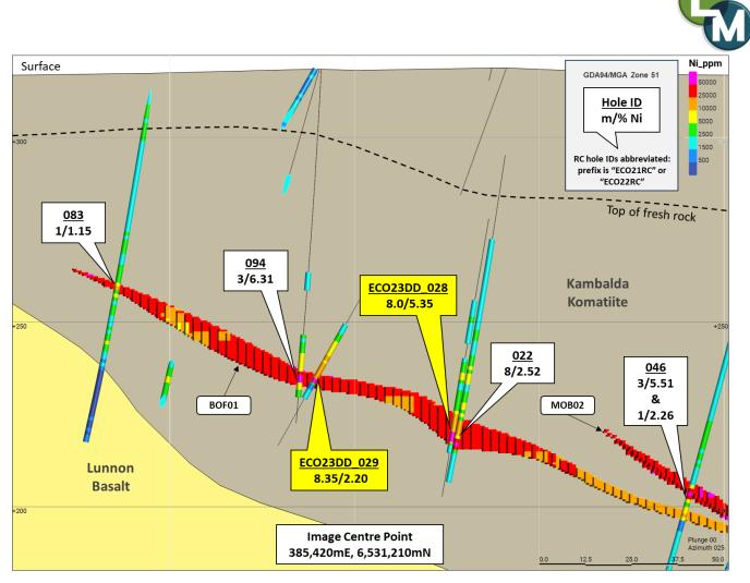
**Figure 2**: Cross section (looking NNE) through the BOF01 domain of the Baker nickel deposit illustrating the drill traces of the reported DD holes (yellow call outs) and their "twin" RC holes (Previous hole ID suffixes, where abbreviated, are "ECO21RC\_" or "ECO22RC\_").
