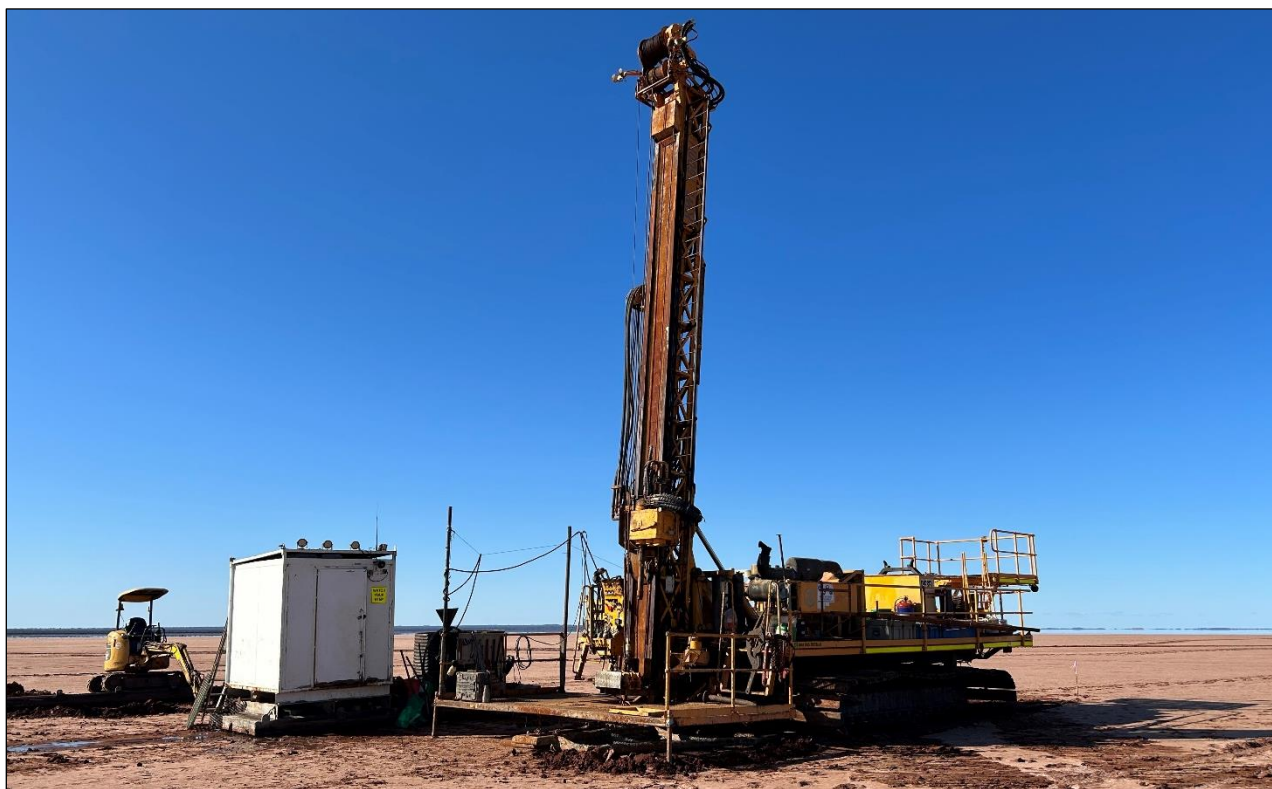
Figure 1: Track mounted, lake-based rig setting up to commence drilling of the Long South Gap prospect – August 2023.
