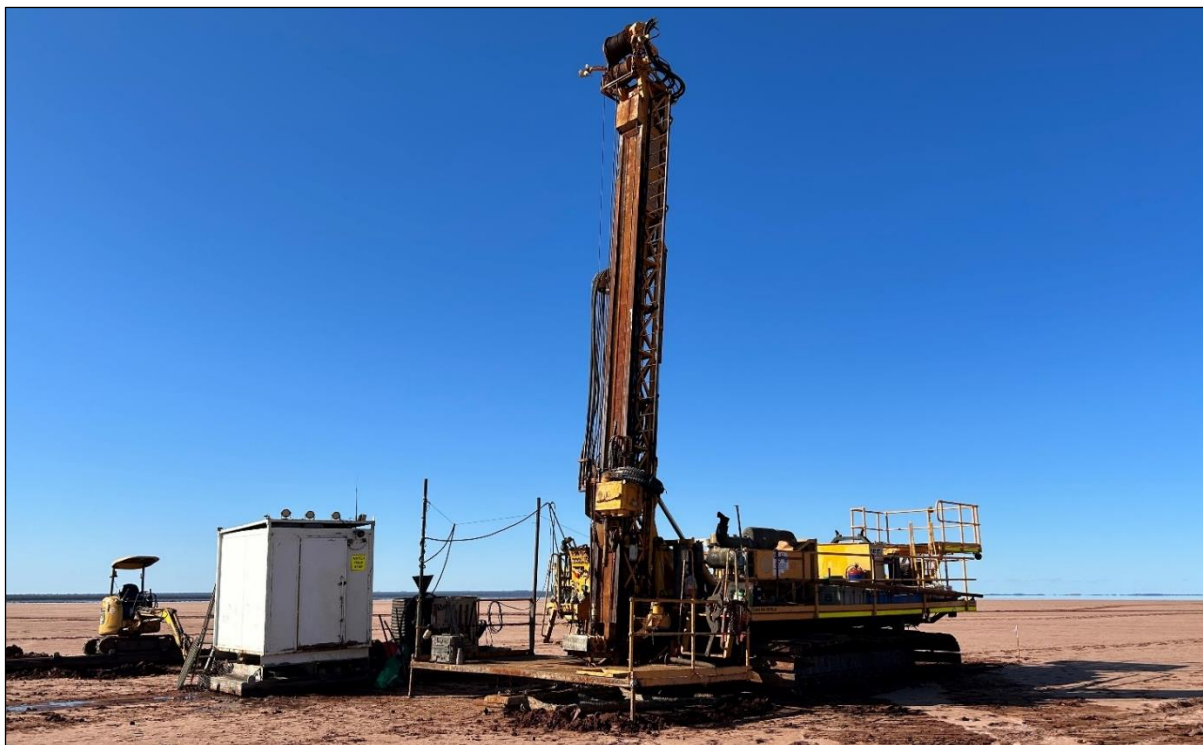
Figure 5: Track mounted, lake-based rig setting up to commence drilling of the Long South Gap prospect – August 2023.
