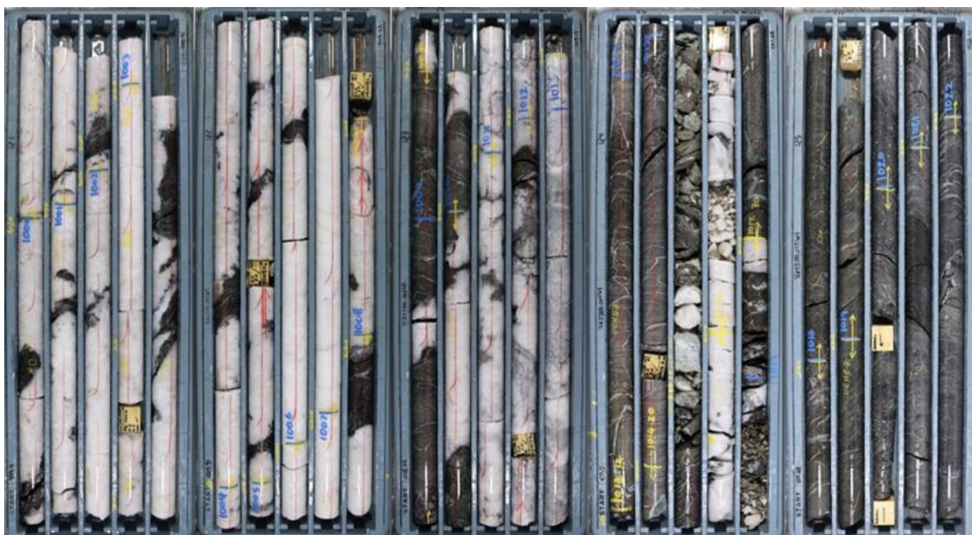
Figure 5: Portion of a broad, gold-bearing structure encountered in SLK23DD_005W1; close to the interpreted prospective nickel contact in the Company's first ever diamond hole at Long South Gap – trays shown 999m to 1,022m downhole depth.
