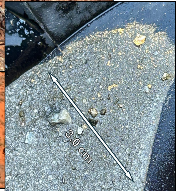
Pan concentrate containing visible gold derived from drill spoil at FOS24RC_056 from the drilled metre which assayed 1m @ 350g/t Au (from 20m) - see ASX announcement dated 10 Oct 2024
