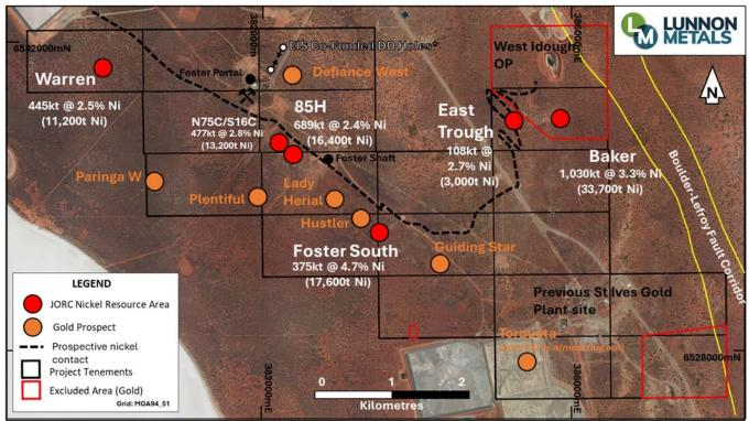
Figure 3: Foster-Baker Project Area showing nickel Mineral Resource<sup>9</sup> positions and select gold prospects.
