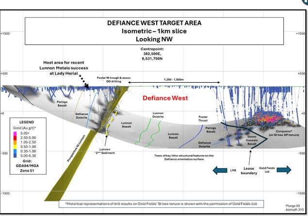
**Figure 6:** 1km thick slice isometric view of Figure 5, draping preliminary litho-structural interpretation on Defiance West structural system (grey surface) and highlighting the absence of drilling testing in the area between Conqueror (Gold Fields Ltd) and Foster nickel mine (Lunnon Metals).
