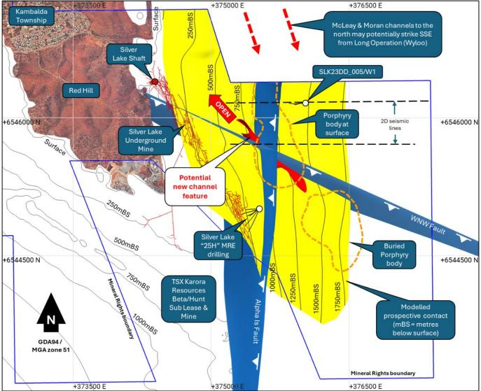
**Figure 8**: Plan view of the Silver Lake-Long South Gap area illustrating geological solid interpretation of the prospective nickel contact, original 2D seismic lines, the 3km long Silver Lake (Lunnon) channel/mine and the location of a newly identified possible new channel interpreted from the 'Cube'.
