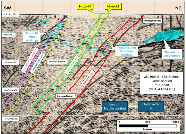
**Figure 5:** 2D Victory Seismic Line<sup>6,7</sup> through the target area looking NW showing SW dipping stratigraphy and Foster Thrust and interpreted flat lying features (structures) between the Foster nickel mine and the Conqueror gold orebody.
