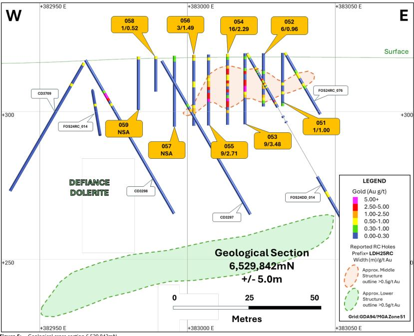
Figure 5: Geological cross section 6,529,842mN
