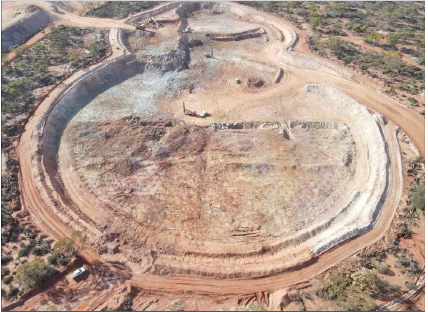
Figure 2: End of March 2026 - mining the Lady Herial Pit 315-310mRL & commenced drilling & blasting 305 RL bench.
