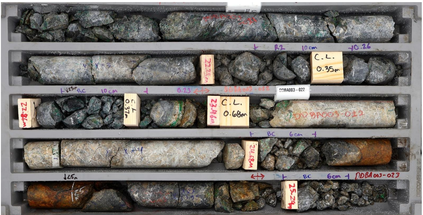
Figure 4: DDBA26-003 21.56-25.35m down-hole. Example of drill core from the Baird Project showing shifts in alteration intensity and mineral distribution across depth. The cores range from relatively fresh grey dolomite into sections marked by green malachite alteration, fracture networks, and subtle bleaching. Mineralized zones appear along veinlets and broken core surfaces, where copper sulphides such as chalcopyrite, chalcocite and bornite accumulate. Secondary copper minerals malachite, chrysocolla and minor azurite present as thin coatings along fractures, reflecting late-stage oxidizing fluids. The combination of veining, alteration, and structural breaks illustrates how copper-rich fluids migrated through the rock column, depositing sulphides preferentially along permeable and structurally prepared zones.
