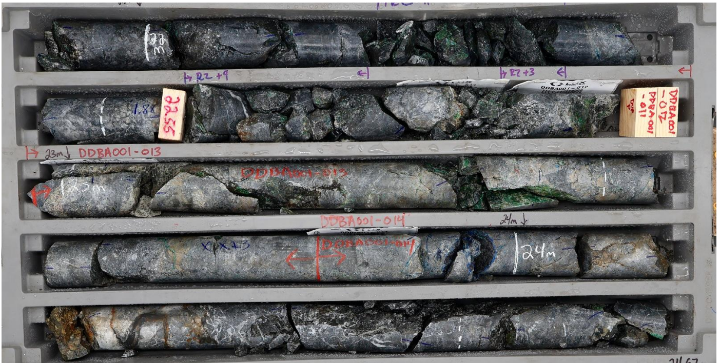
Figure 3: DDBA26-001 21.9-24.67m down-hole. Example of drill core from the Baird Project highlighting the shifts in alteration style and mineralogy down-hole. The cores display a progression from dark grey, relatively unaltered carbonate sediment into intervals marked by greenish malachite alteration and subtle veining. Fine fractures and veinlets host pale to dark green copper minerals representing disseminated chalcopyrite, bornite, and secondary copper carbonates and silicates along fracture surfaces. These mineralized zones coincide with increased fracturing and changes in rock fabric, reflecting the pathways of copper-rich hydrothermal fluids.
