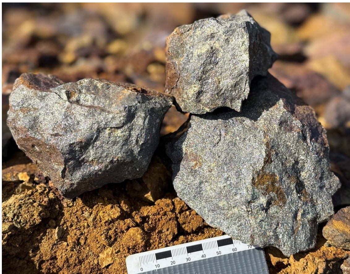
Figure 7: | Skyfall Prospect - Outcrop sample M209550 chalcopyrite rich sulphide sample.
