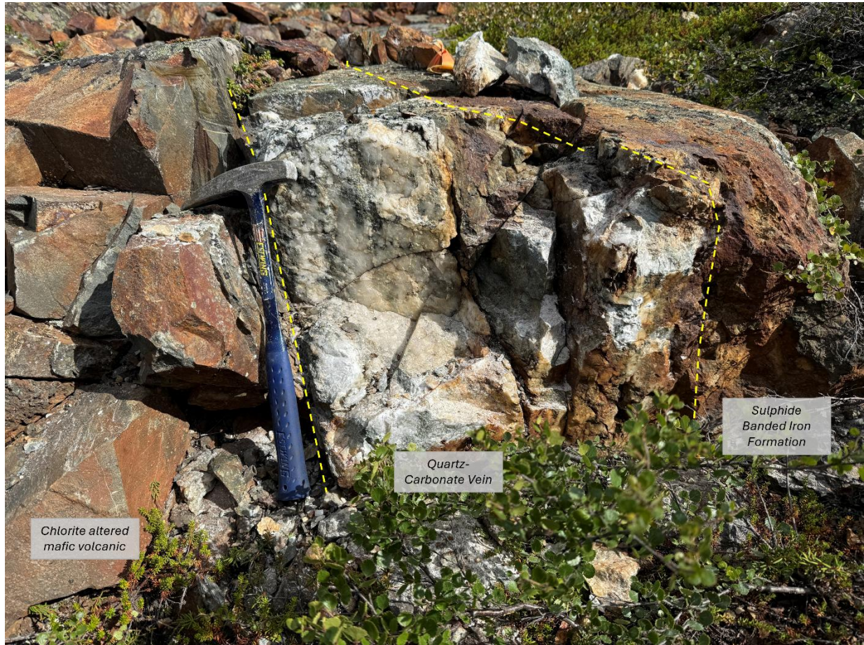
Figure 10: | Defender - Outcrop of quartz carbonate vein at the contact between chlorite altered mafic volcanics and sulphide BIF. Location of sample M209567.
