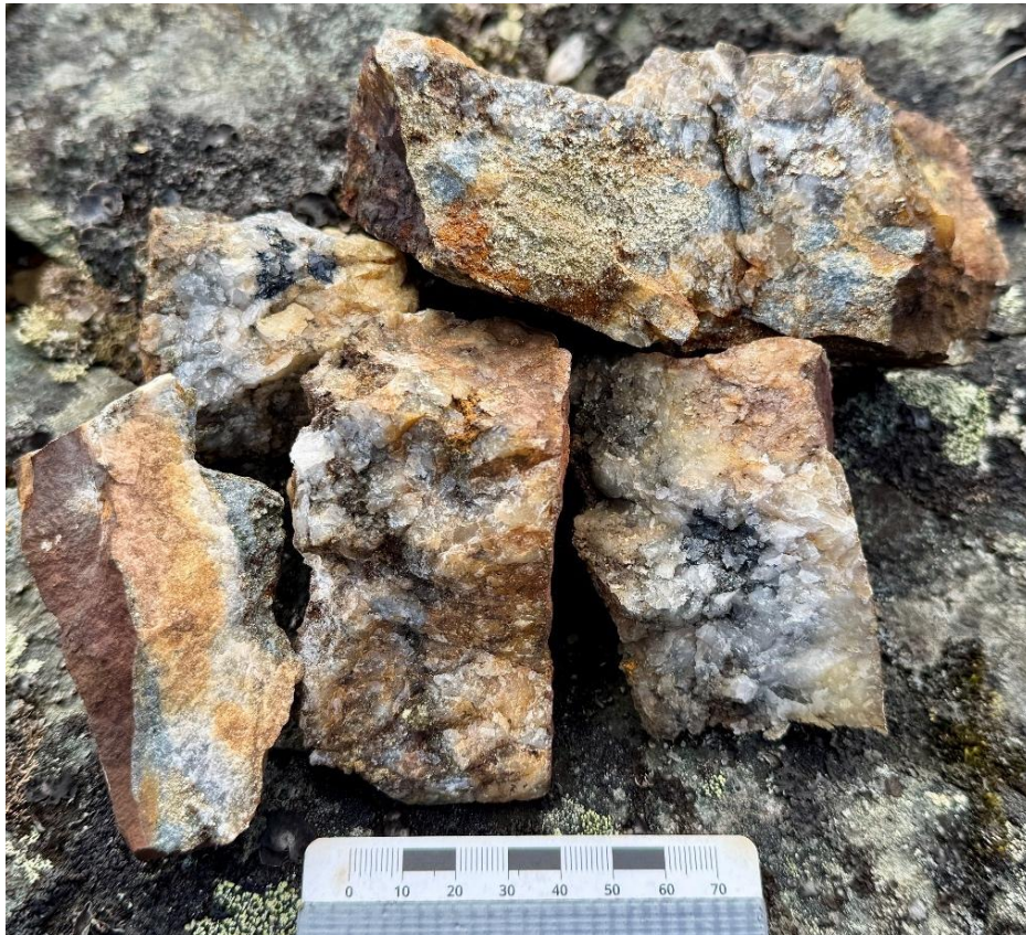
Figure 5: | Quantum Sample M209538. A quartz-pyrite-chalcopyrite-galena vein.
