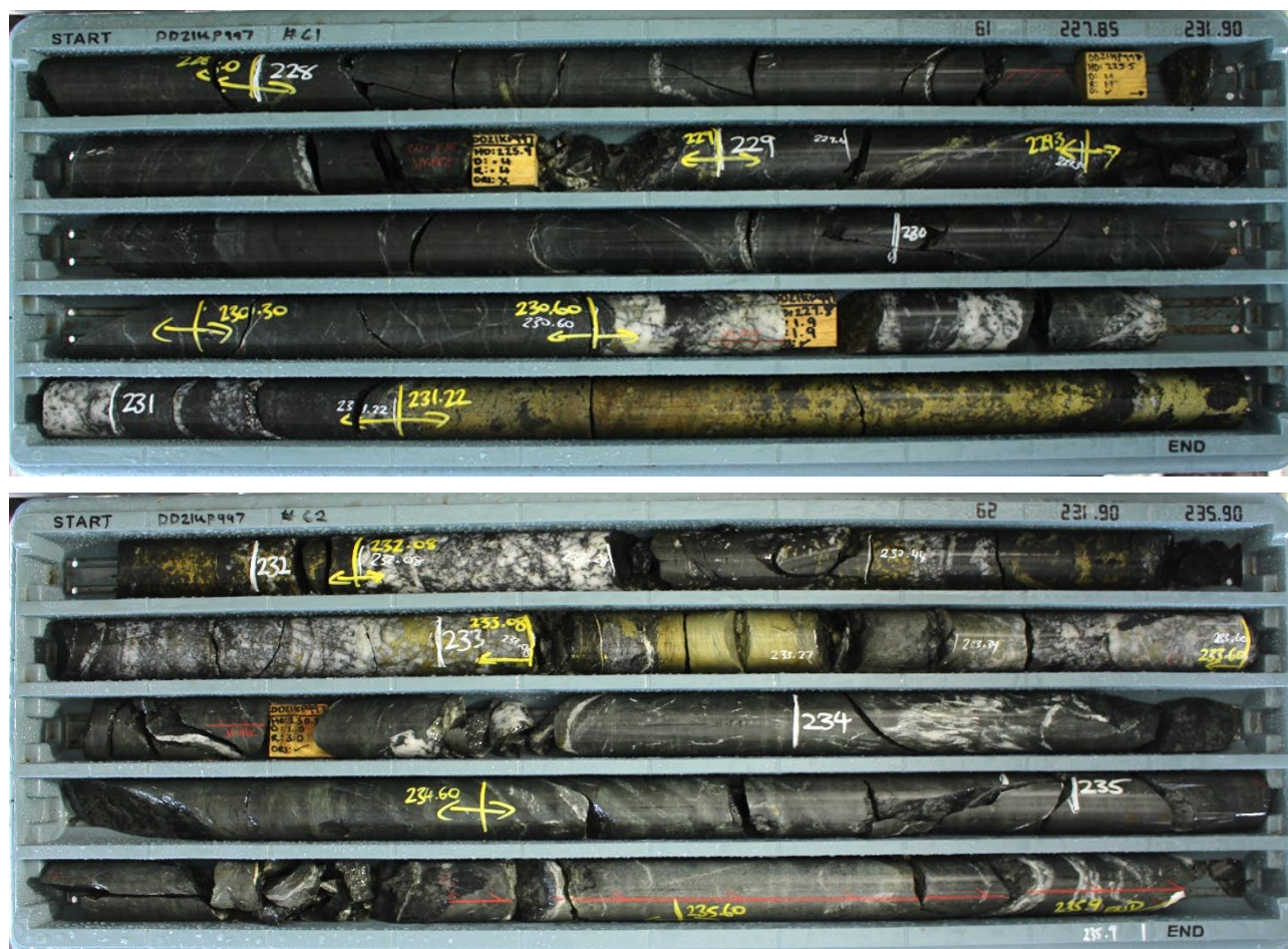
Figure 2: DD21KP997 at Harbour View South. Reported intercept commencing at 231.22m down hole.
