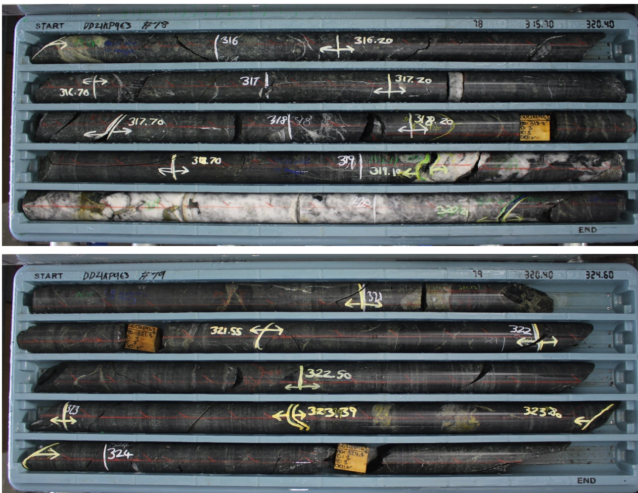
Figure 9: DD21KP963 with the ~10cm shallow south dipping quartz-sulphide vein at 321.05m in the footwall to a larger quartz-sulphide west dipping vein.
