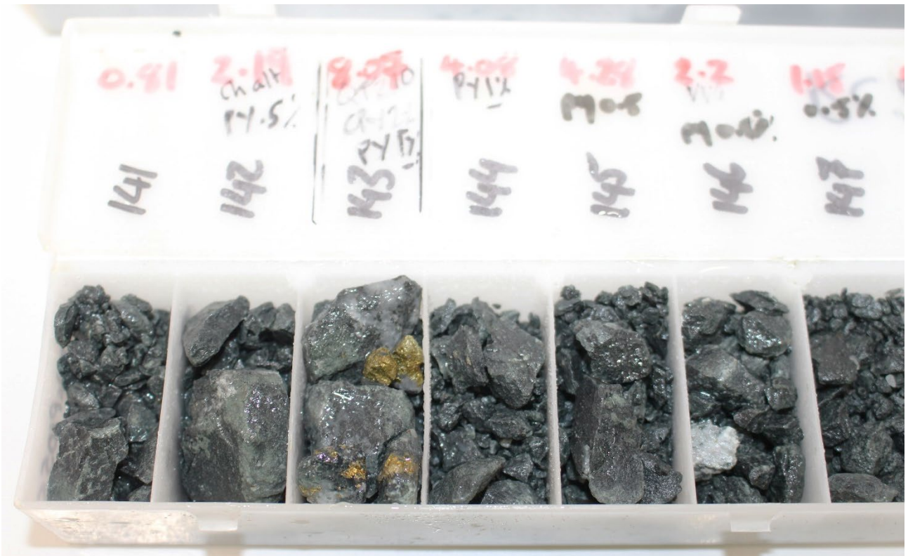
Figure 7: Mineralisation within RC21KP1055 with 0.5% – 1% pyrite surrounding quartz-sulphide (pyrite-chalcocopyrite) vein with 1m @ 8.07 g/t Au, 0.23 % Cu, 0.6 g/t Au from 142m.
