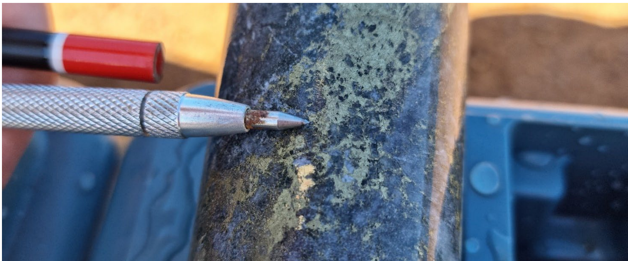
Figure 3: DD21KP1033: quartz-pyrrhotite-chalcopyrite mineralisation with visible gold approximately 102m downhole
