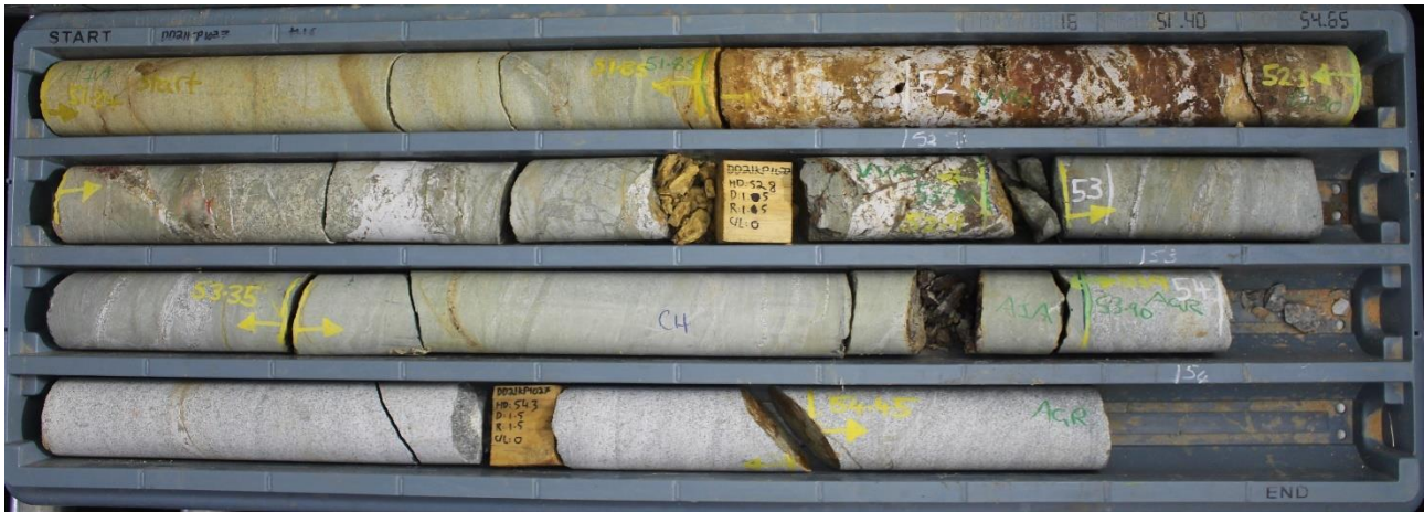
Figure 8: Gossanous textured quartz-hematite-goethite veining within DD21KP1027 at the eastern end of Gem. Mineralisation includes 0.45m @ 27.8 g/t Au, 0.32 % Cu, 25.3 g/t Ag from 51.85m. Nuggety gold within the oxide is inferred with less than detection gold values between 52.3m-52.9m that is also host to 1.41% Cu and 12 g/t Ag including native copper.
