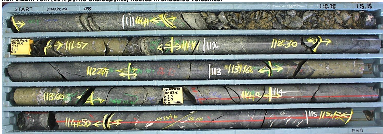
Figure 7: Twin massive sulphide (85% pyrite, 15% chalcopyrite) veins in DD21KP1028 from 111.57m and 113.16m respectively with blebby ~5% sulphides between. Veins are hosted in the tonalite.
