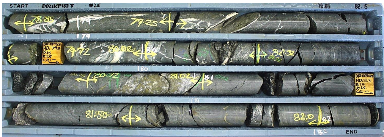
Figure 6: 0.7m interval grading 24.06 g/t Au from 80.32m within DD21KP1028. Geology of the interval consists of a sulphide rich 0.22m vein (50% pyrite-chalcopyrite) hosted in andesitic volcanics.
