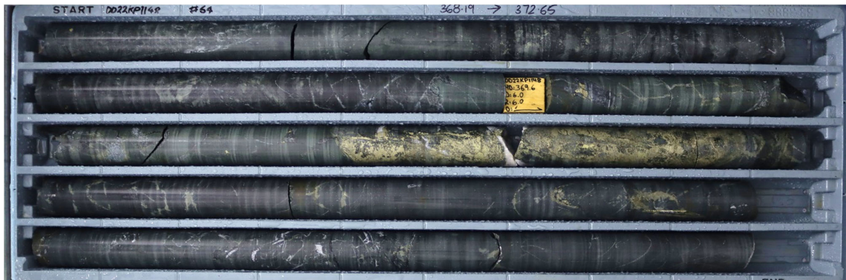
Figure 6: DD22KP1148 sulphide dominant vein between 370.3m - 370.8m. Sulphide consists of pyrite 50% and chalcopyrite (5%). Approximately 5% sulphide stringer veins persist for an additional 1.5m into the footwall of the vein.
