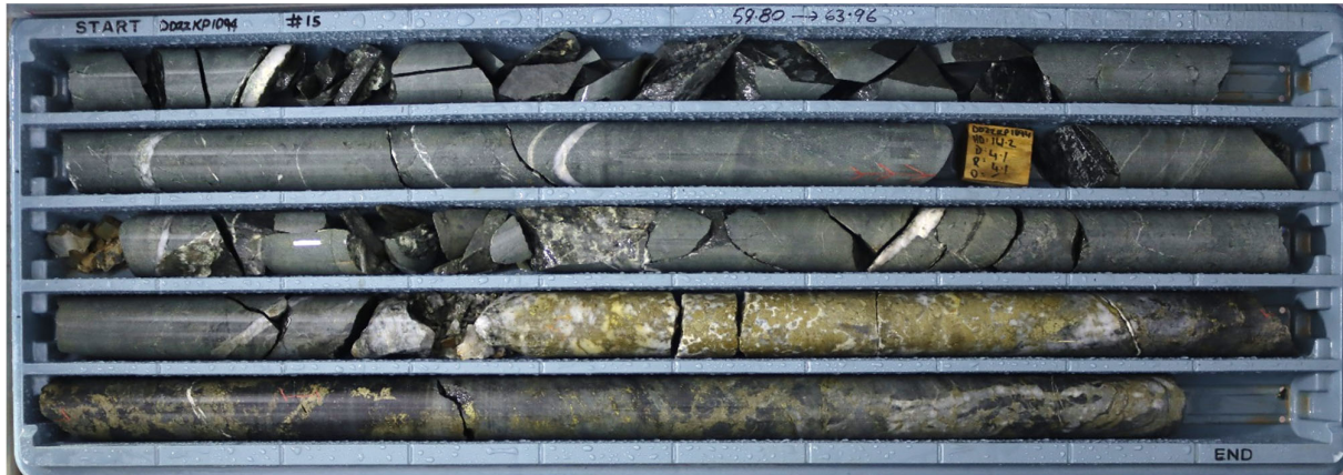
Figure 4: DD22KP1094 highlighting quartz-sulphide veining between 162.6m – 164.65m with associated dark green chlorite alteration.
