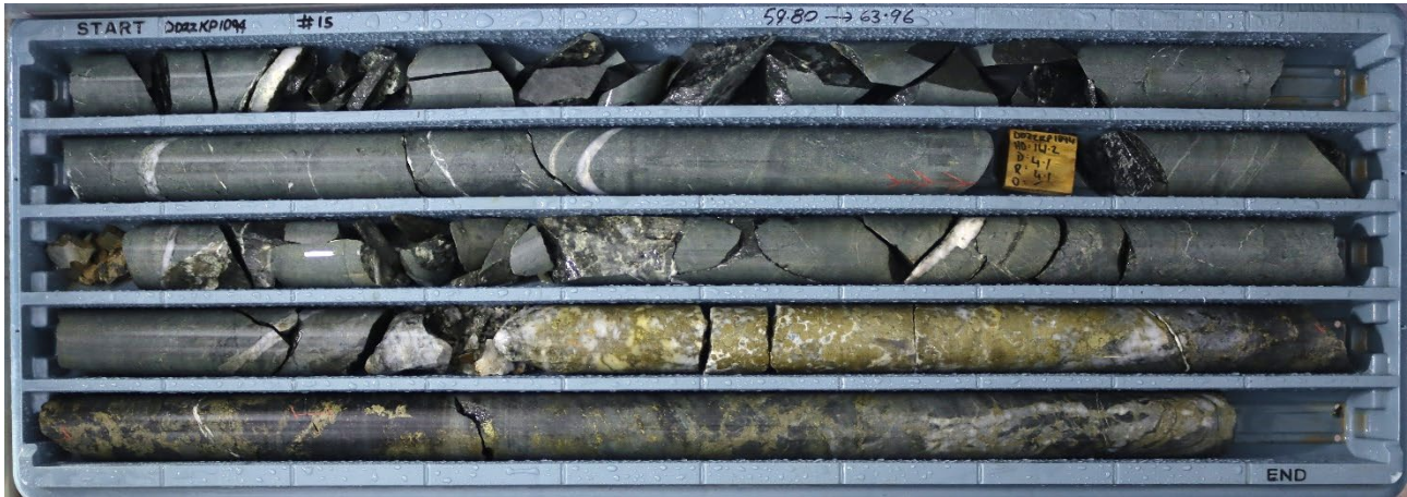
Figure 4: DD22KP1094 highlighting quartz-sulphide veining between 162.6m – 164.65m with associated dark green chlorite alteration. Total sulphide abundances estimated at 60% comprised of 20% chalcopyrite and 40% pyrite.
