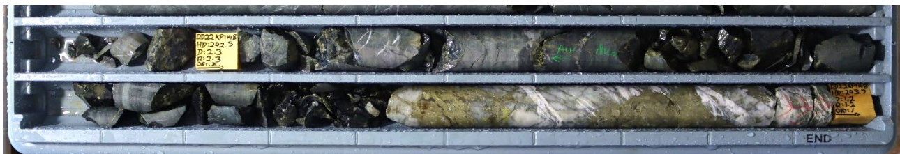
Figure 4: DD22KP1094 highlighting quartz-sulphide veining between 162.6m – 164.65m with associated dark green chlorite alteration. Total sulphide abundances estimated at 60% comprised of 20% chalcopyrite and 40% pyrite.
