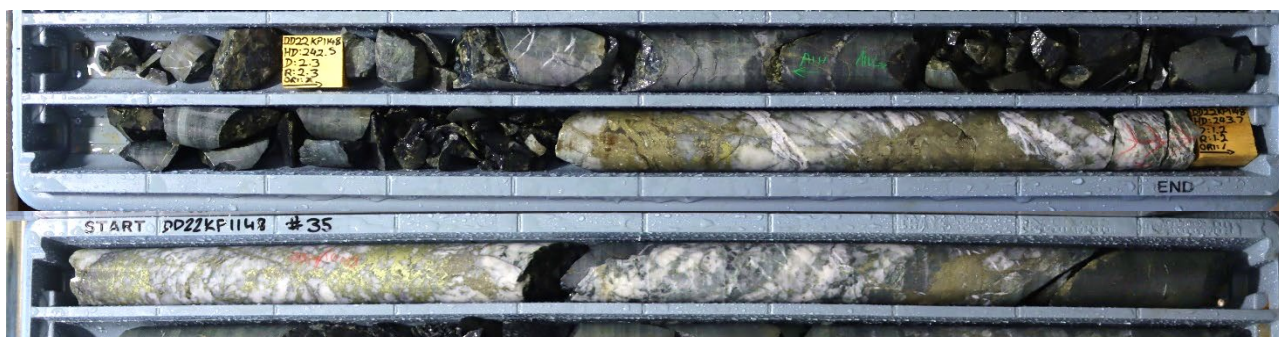
Figure 1: DD22KP1148 with quartz-pyrite-chalcopyrite veining at approximately 243m downhole.
