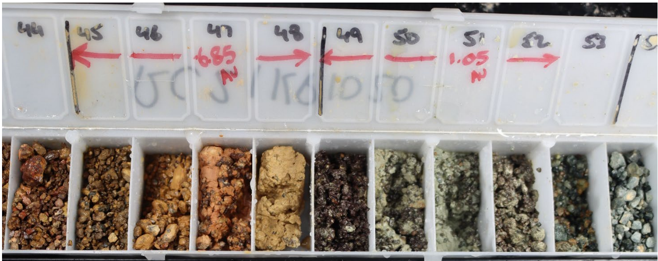
Figure 6: Oxidised quartz-gravel and clays within RC21KP1020 situated at the contact with saprock. Composite grades are written on chip trays. 1m re-splits of samples recorded 2m @ 7.89 g/t Au, 0.19 % Cu, 0.35 g/t Ag from 44m including 1m @ 14.40 g/t Au from 44m.
