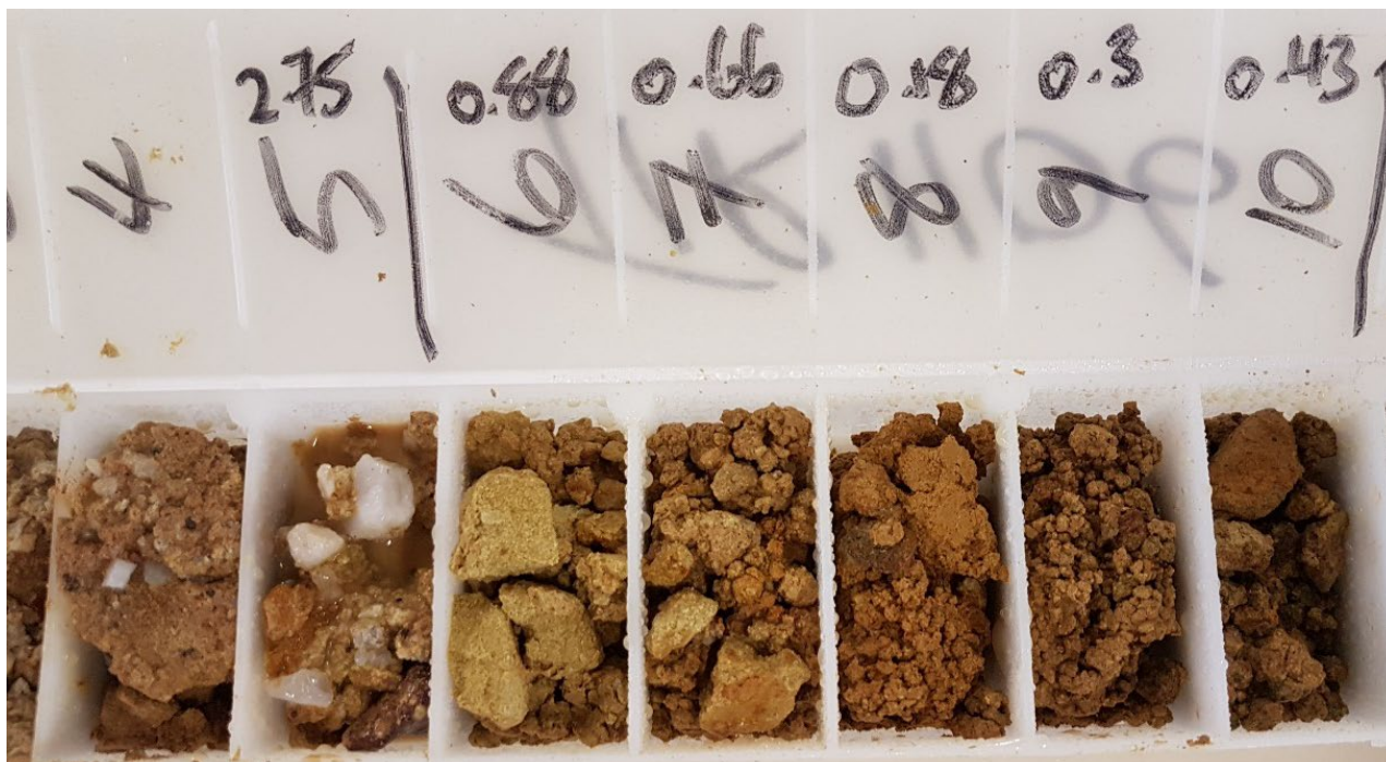
Figure 5: Aircore hole TTR1065 at Gift South. Quartz clasts of the mineralised horizon (4-5m interval) are dominant over clays. Lower grade intervals within intense brown clays (5m-10m) are observed.
