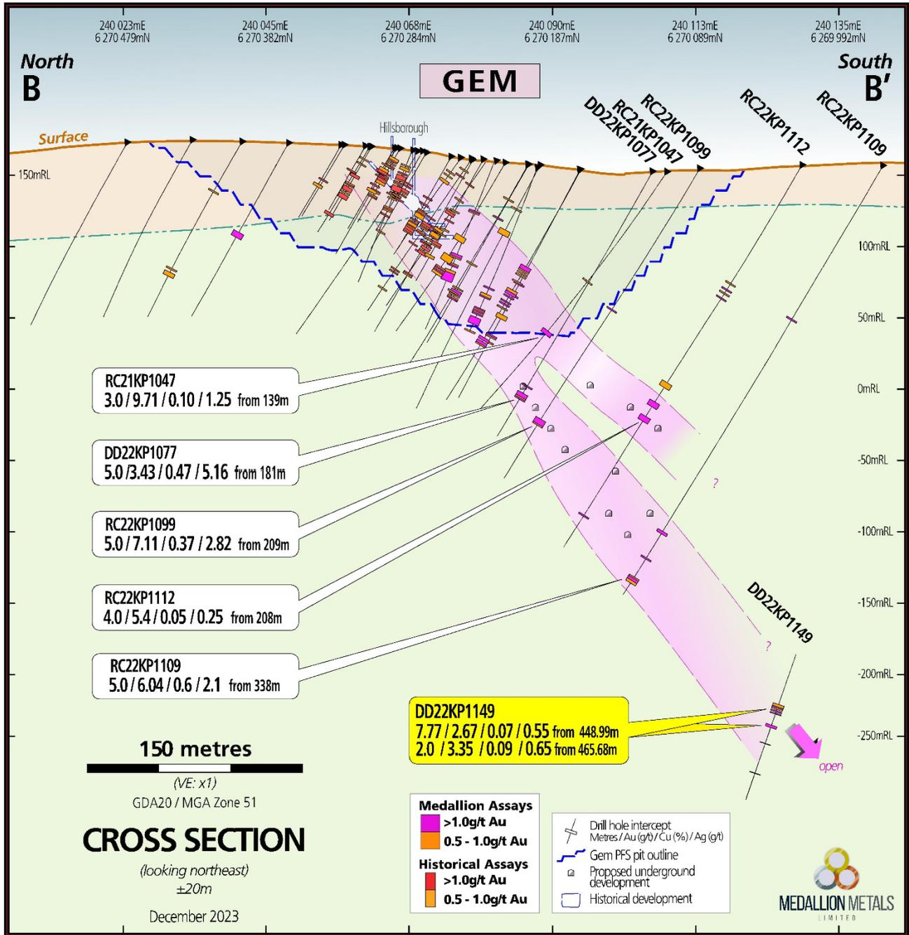
Figure 4: Cross section B-B' (refer to Figure 1 for section location) through the Hillsborough lodes with recent drilling results. DD22KP1149 represent the deepest hole drilled at Gem, 140m down plunge from RC22KP1109.
