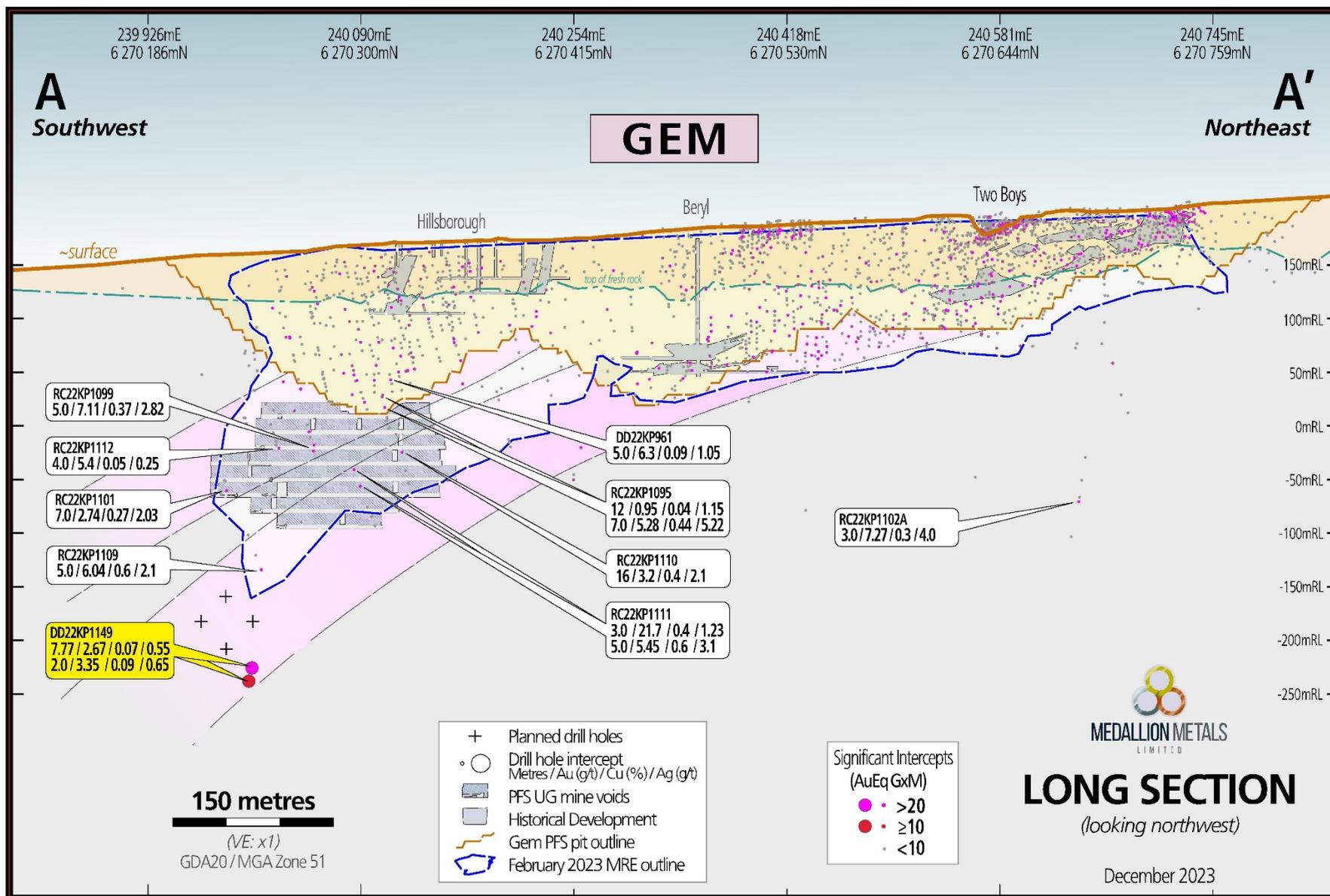
Figure 3: Long section view of Gem showing drill results relative to previous drilling and current MRE extents (see Figure 1 for location of section line A-A').
