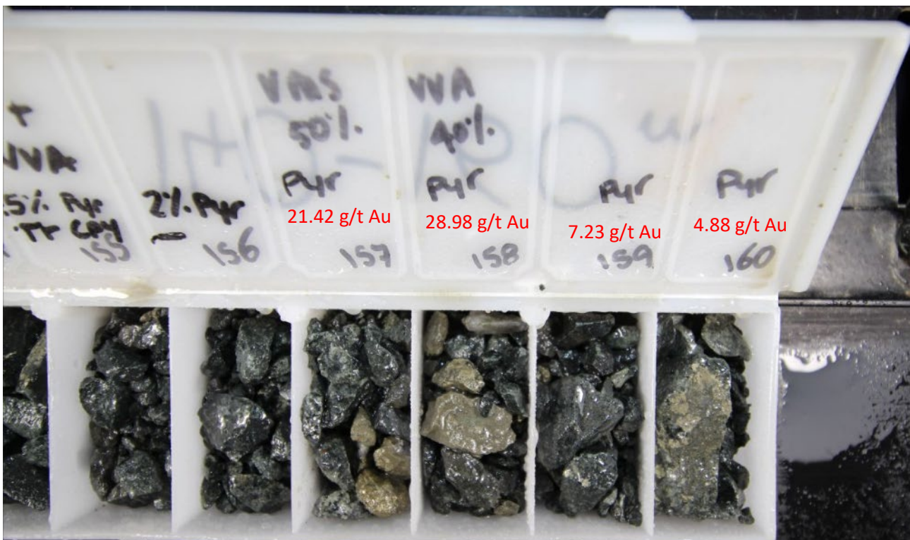
Figure 3: R22KP1205A intersected 4m @ 15.60 g/t Au, 0.7 % Cu, 12.2 g/t Ag from 156m. Mineralisation associated with the high-grade lode is predominantly sulphides, 10-40% Pyrite and trace chalcopyrite, and minor quartz veining.
