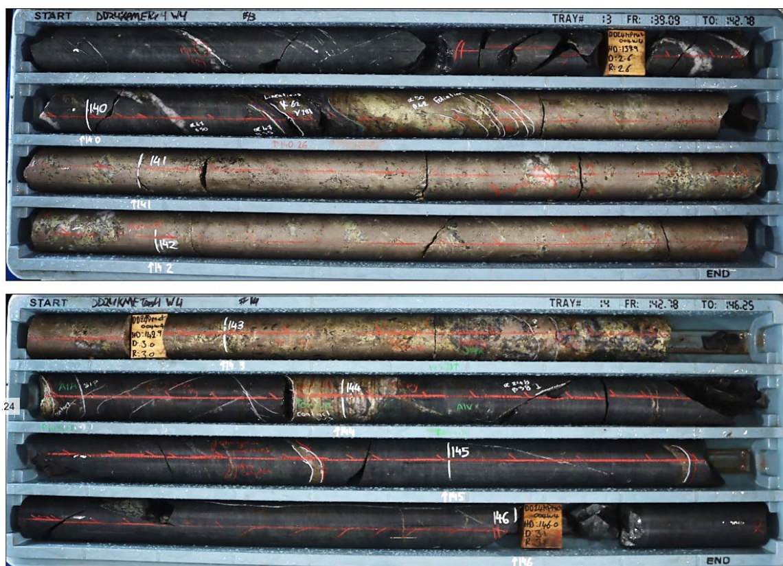
Figure 6: DD24KPMET004_W4 – 3.90m zone containing semi massive - massive sulphide and quartz-sulphide vein from 139.70m, comprised of ~45% pyrrhotite, ~35% pyrite, ~15% chalcopyrite, 5% quartz.
