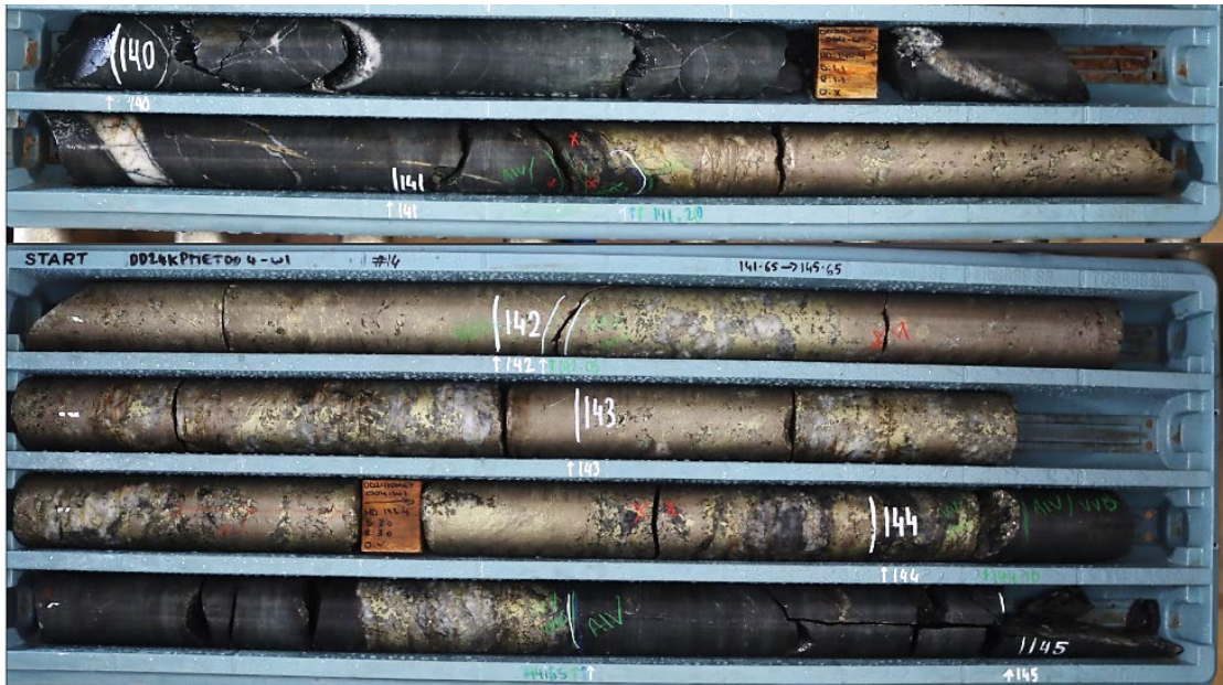
Figure 3: DD24KPMET004_W1 – 3.45m zone containing semi massive - massive sulphide and quartz-sulphide vein from 141.20m, comprised of ~40% pyrrhotite, ~35% pyrite, ~15% chalcopyrite, 10% quartz.
