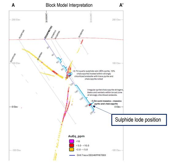
Figure 3: DD24KPMET003 in cross section. The plan location and orientation of the cross section is provided in Annexure 1.
