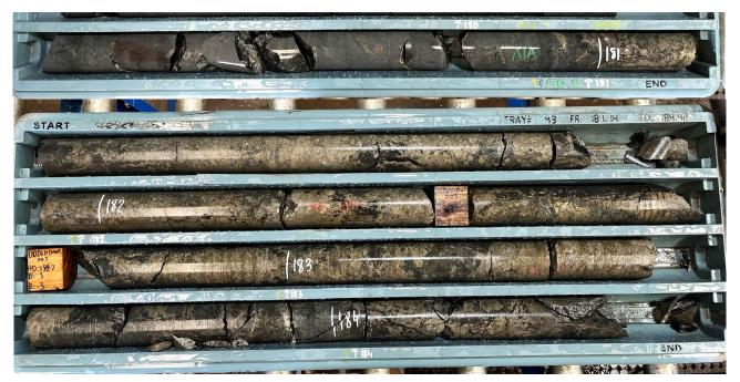
Figure 1: DD24KPMET003 displaying semi massive to massive pyrite-chalcopyrite mineralisation from approximately 181m downhole (assays pending).
