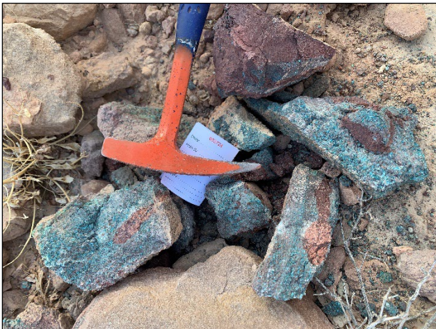
Figure 4: Sampled outcrop of copper bearing target formation; 7.45% Cu (Sample 003724); Um el Amad mine
