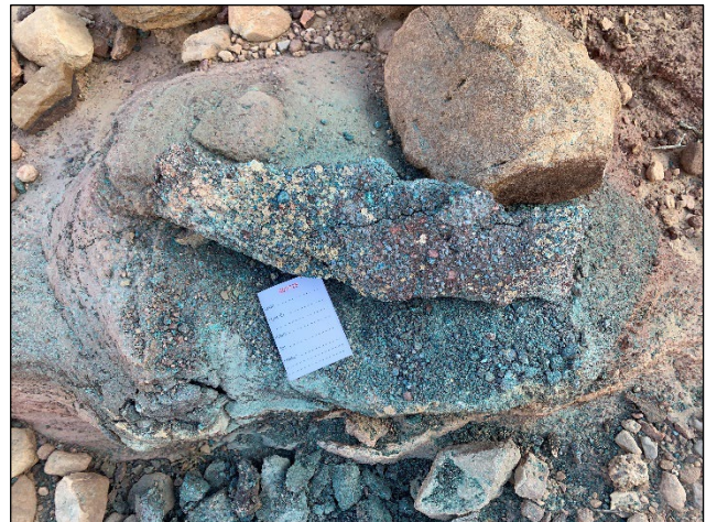
Figure 5: Sampled outcrop of copper bearing target formation; 8.69% Cu (Sample 003725); Um el Amad mine
