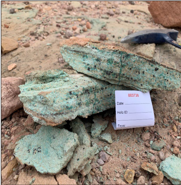
Figure 6: Mineralised sandstone, Um el Amad mine region. 2.51% Cu.
