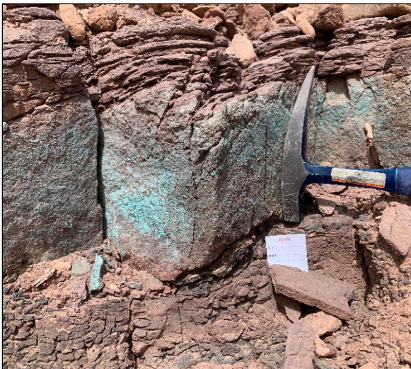
Figure 8: Mineralised sandstone, Malaqa NW. 6.25% Cu.
