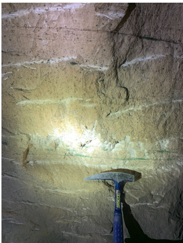
Figure 3: Underground mine face showing disseminated, blebby to streaky Cu in fine sandstone/dolomite. Um el Amad mine.
