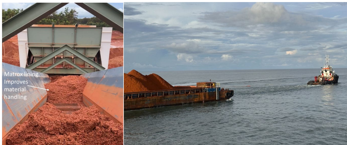
Pictures: Left: New, low friction Matrox lining boards fitted to the Apron Feeder to enhance throughput rates and reduce blockages. Right: Mandang pulling a loaded bauxite barge.
