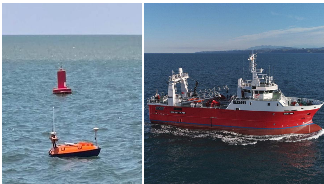
Pictures: (L) New marine survey drone being used to assist bed levelling campaign (R ) Specialised bed-levelling tug Destiny.
