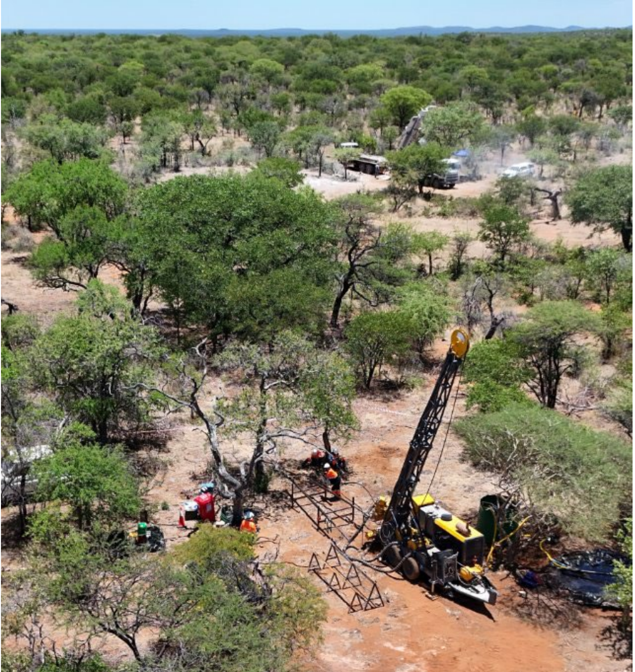
Photo 1: RC (background) and diamond (foreground) drilling at T-13 Deposit, Otavi Project.
