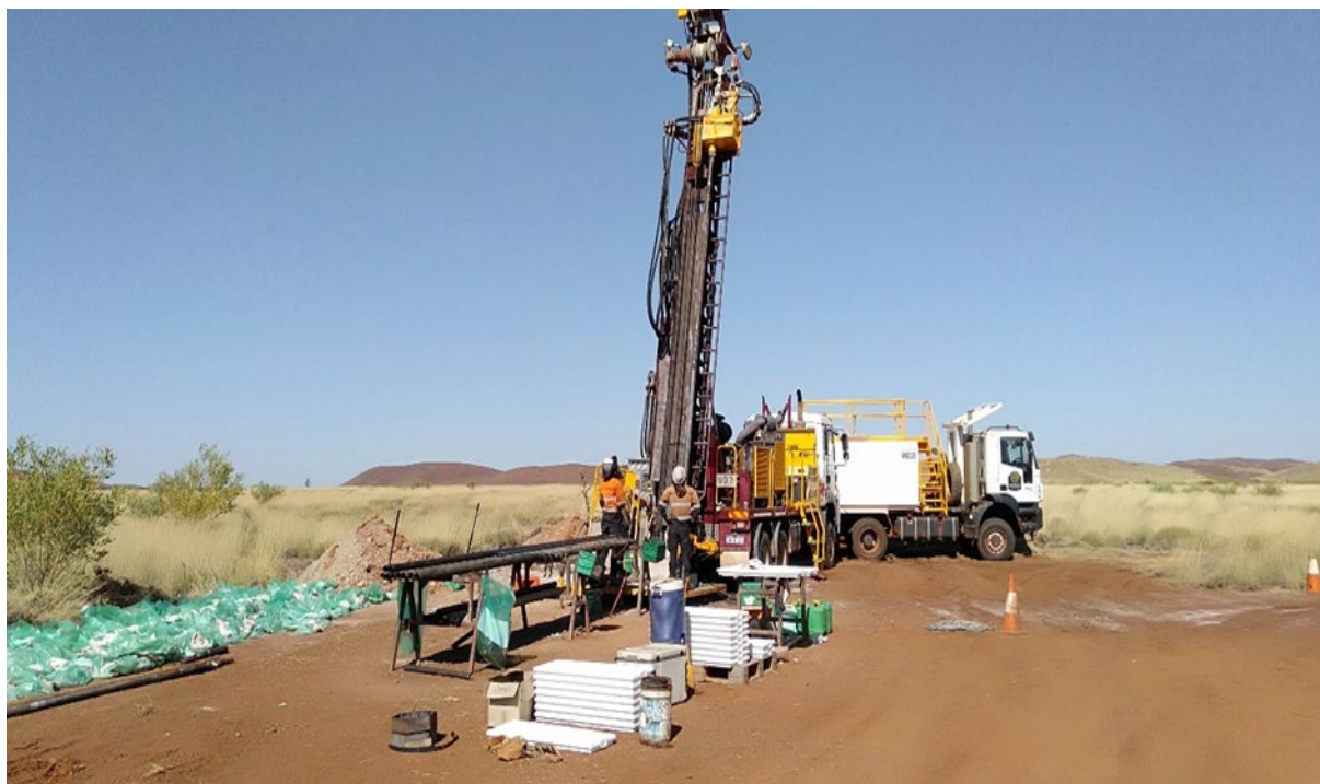
Figure 2 – Diamond Core Drill Rig on drill hole M22_001_RCD
