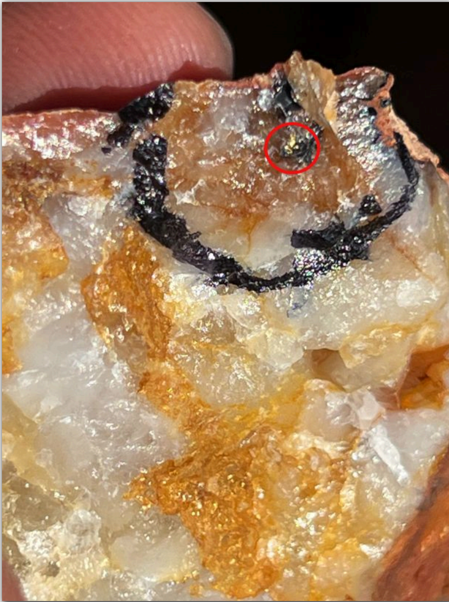
Picture 2: Picture Showing Gold in Quartz from RI 402m in the SE Corner of the Bulk Sampling Area
