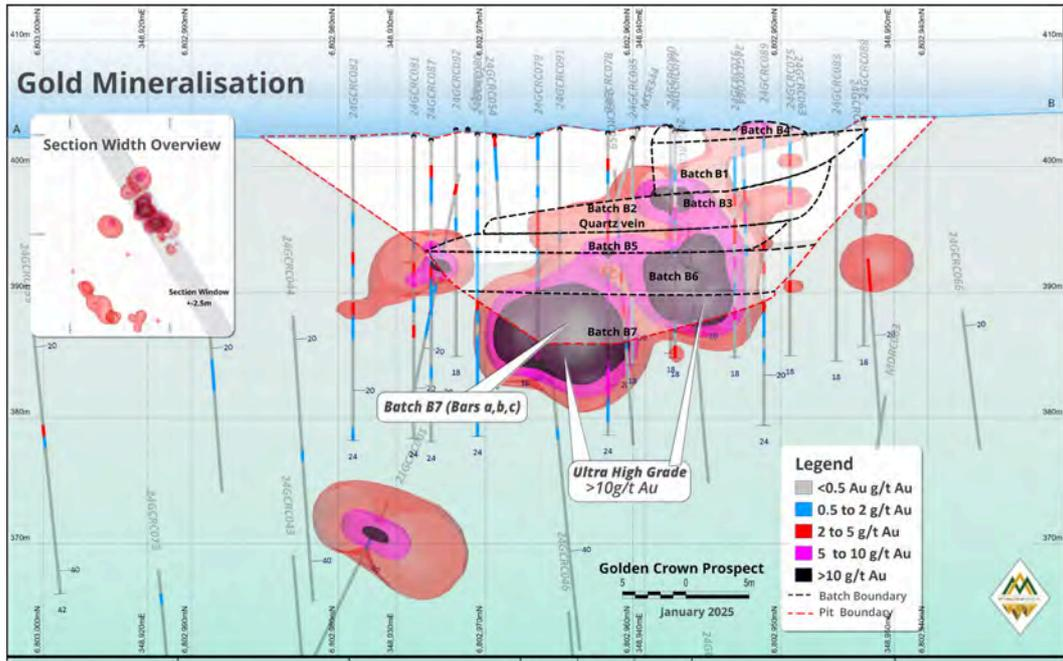
Figure 2: Long Section along the central part of the Golden Crown bulk sampling area, drillholes collars, Au values and depth of batches marked on the section.
