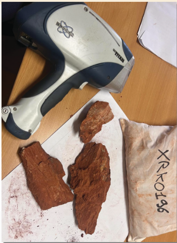
Picture 1: Rock Chip XRK0196 Ferruginous Copper Gossan
