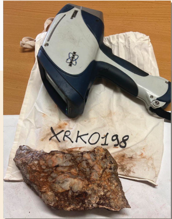
Picture 2: Rock Chip XRK0198 Quartz hydrothermal Breccia with Iron Oxide alteration
