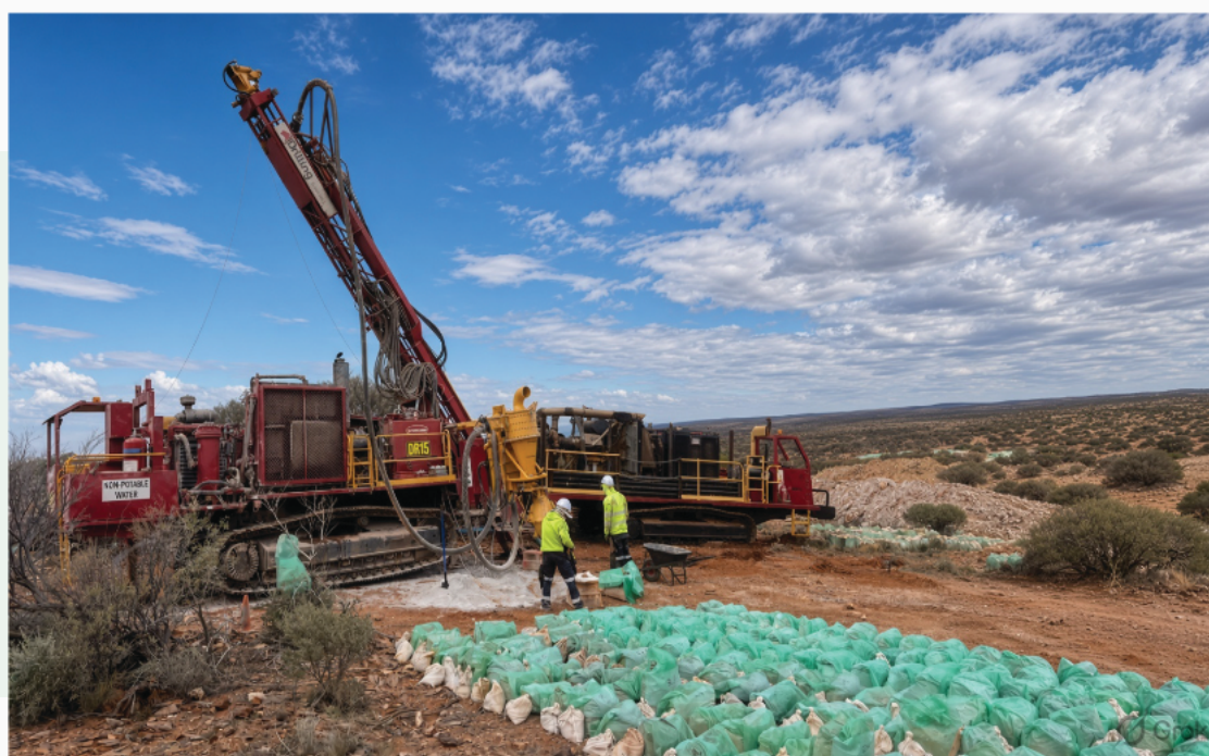
Figure 11: Track-mounted RC rig of the type used for the program (shown at the latest Golden Crown drilling)
