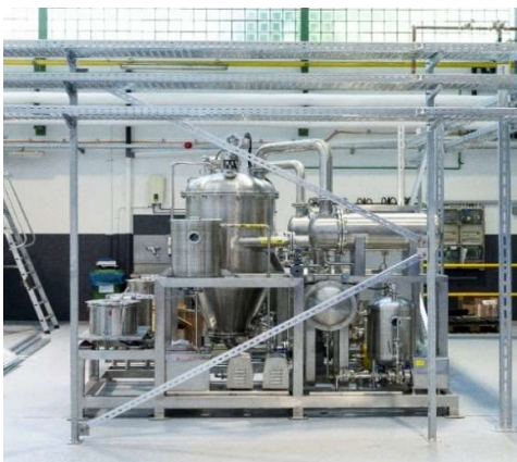
Figure 10 – Final Product Crystalliser.
