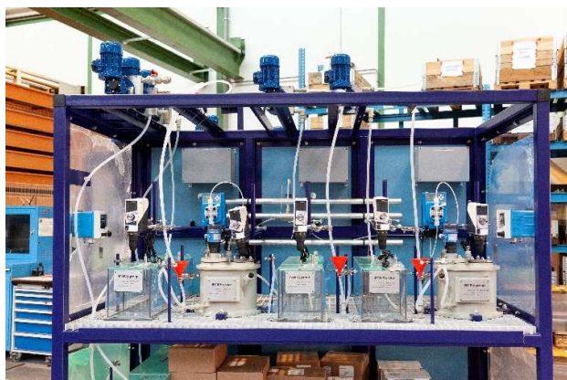
Figure 9 – Single Solvent Extraction Mixer/Settler Circuit
