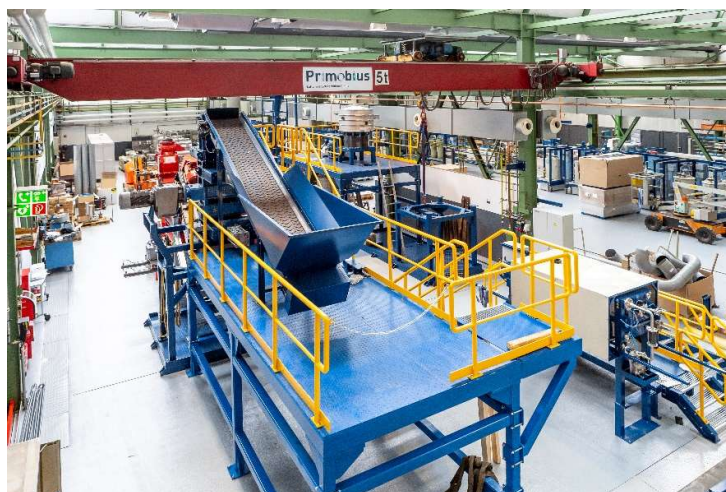
Figure 1 – Two stage Shredding Circuit
