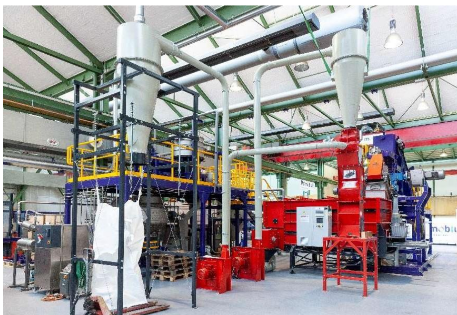
Figure 3 - Shredder feeding into Primary Classification Circuit (foreground - red) removes and bags plastics and Cu/Al metal foils
