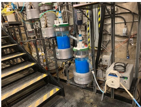
Figure 5 - Copper Crystallisers (left) and Copper Sulphate Product Filter (right)
