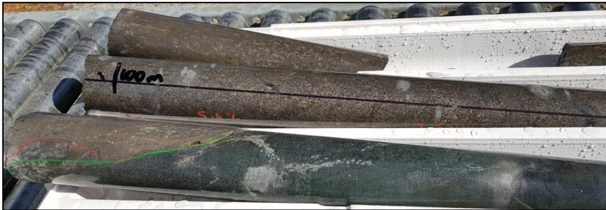
Figure 10 – Photo of diamond core from drill hole EMD002. Massive Nickel Sulphide (grading 6.11% Nickel) is clearly identifiable above a sharp contact with the underlying basalt.
