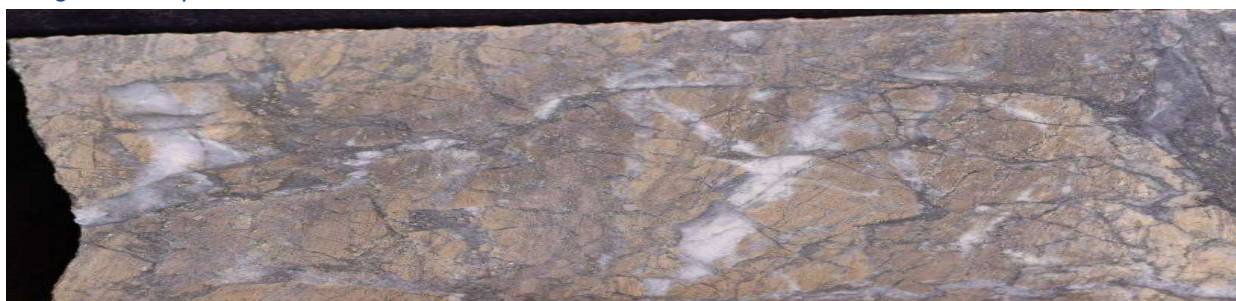
Figure 4b. Mineralised NSD058 asp-cpy-carbonate-sericite altered sulphide-rich interval on the lower margin of interpreted basalt.
